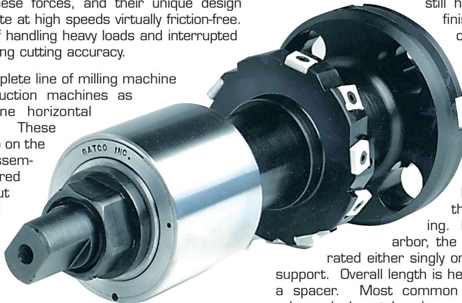
Gatco Anti-Friction Rotary Milling Arbor Bushings are self contained pre-loaded bearing cartridges used to support gang milling arbors. They consist of a stationary outer case; a hardened and ground liner which rotates with the arbor; anti-friction bearings and seals. They are manufactured in several series with each having size and load rating capacities to cover the broadest range of milling applications.
