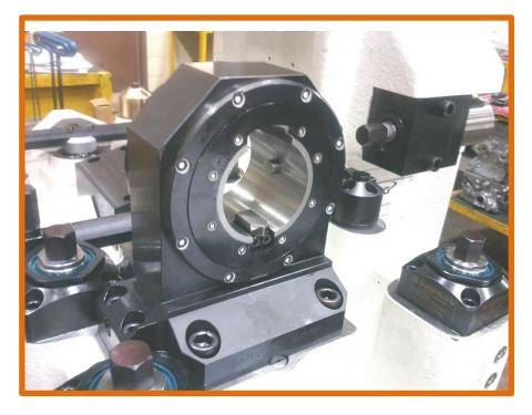
In the evolution of machining technology the automotive industry has been changing their machining practices from dedicated engine lines (transfer lines) to flexible lines. Flexible lines allow the customer to change parts or dimensions at a relatively quick speed and lower cost. Using GFA fixture assemblies allows the user to change the line bar support quickly.
